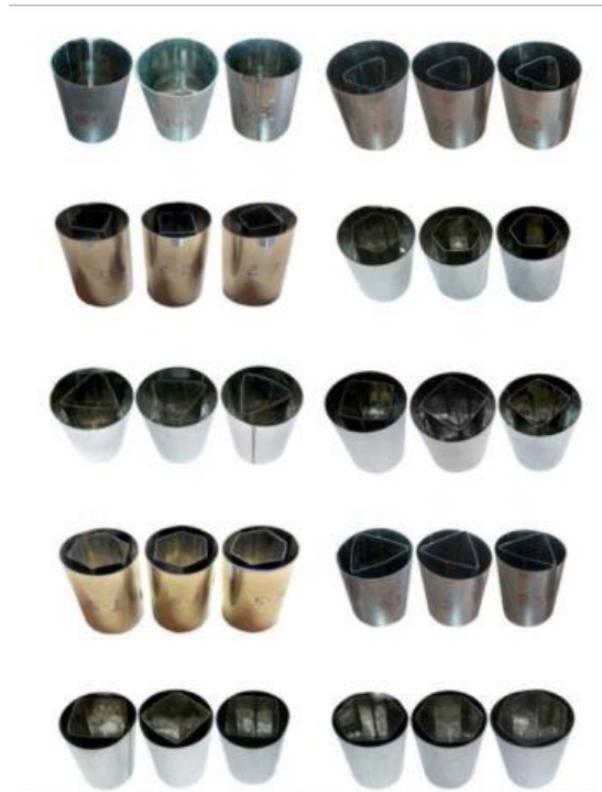
Fig. 1. Bitubular specimens with inner inscribed sections [5].
