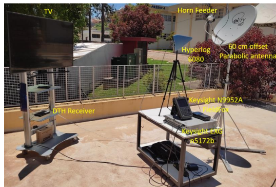
Fig. 1. Proposed setup: a) Block diagram; b) Experimental setup.
