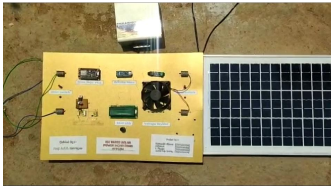
Fig. 2. Hardware Model of Solar monitoring System Using IOT
