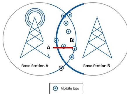
**Fig. 1: Switching of the MN near the edges**
