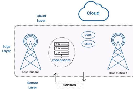
**Fig. 2: Edge computing framework for handover process**
