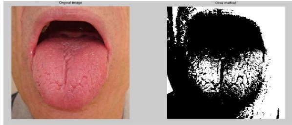
Fig 3.3. The output of Otsu thresholding of the sample tongue image
