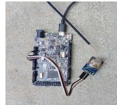
Fig. 10. Testing of MQ2 (Smoke) sensor
