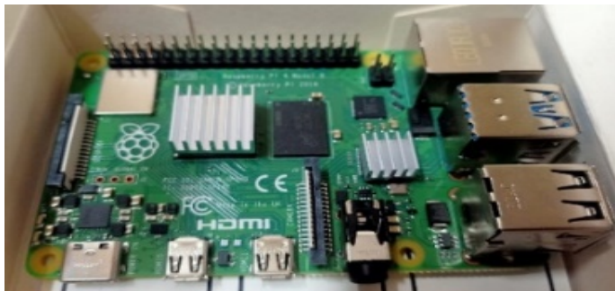
Figure 1. Raspberry Pi 4b.
