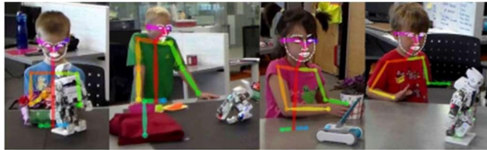
Fig. 2. Facial keypoints and upper body skeleton extracted by OpenPose
