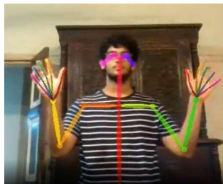
Fig. 6. Openpose Keypoint Detection and Skeleton generation on the Captured Video
