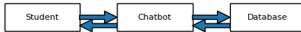
Figure 3. Level 0 Data Flow Diagram that indicates communication between the users and the chatbot system.
